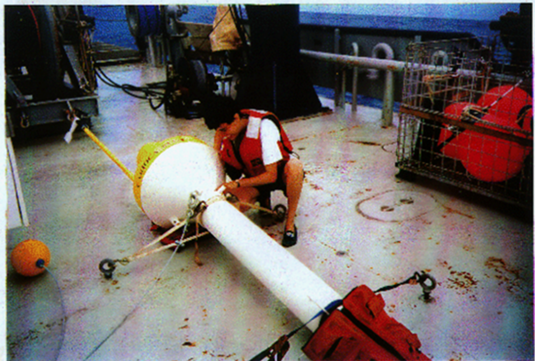
CARIOCA buoy Length:2m Weight:60kg
