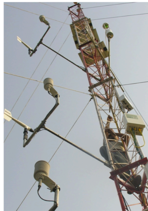
Sunderaban Tower, Sensors shown on different levels
